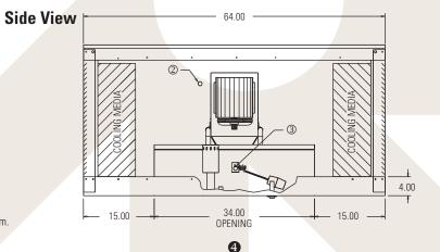
③ 3/8" Compression fitting connection made inside unit.
