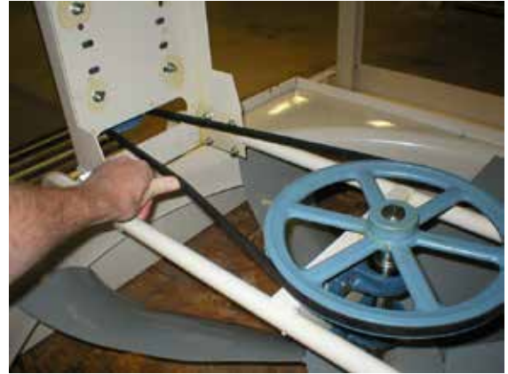
FIGURE 8.1 - Belt Tension - Propeller Fan Coolers Shown
